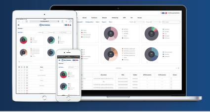
Remote Management System (RMS) enables remote management and monitoring of Teltonika network devices. The system allows you to reconfigure and collect status information from individual network devices even if the devices do not have public IP addresses.
